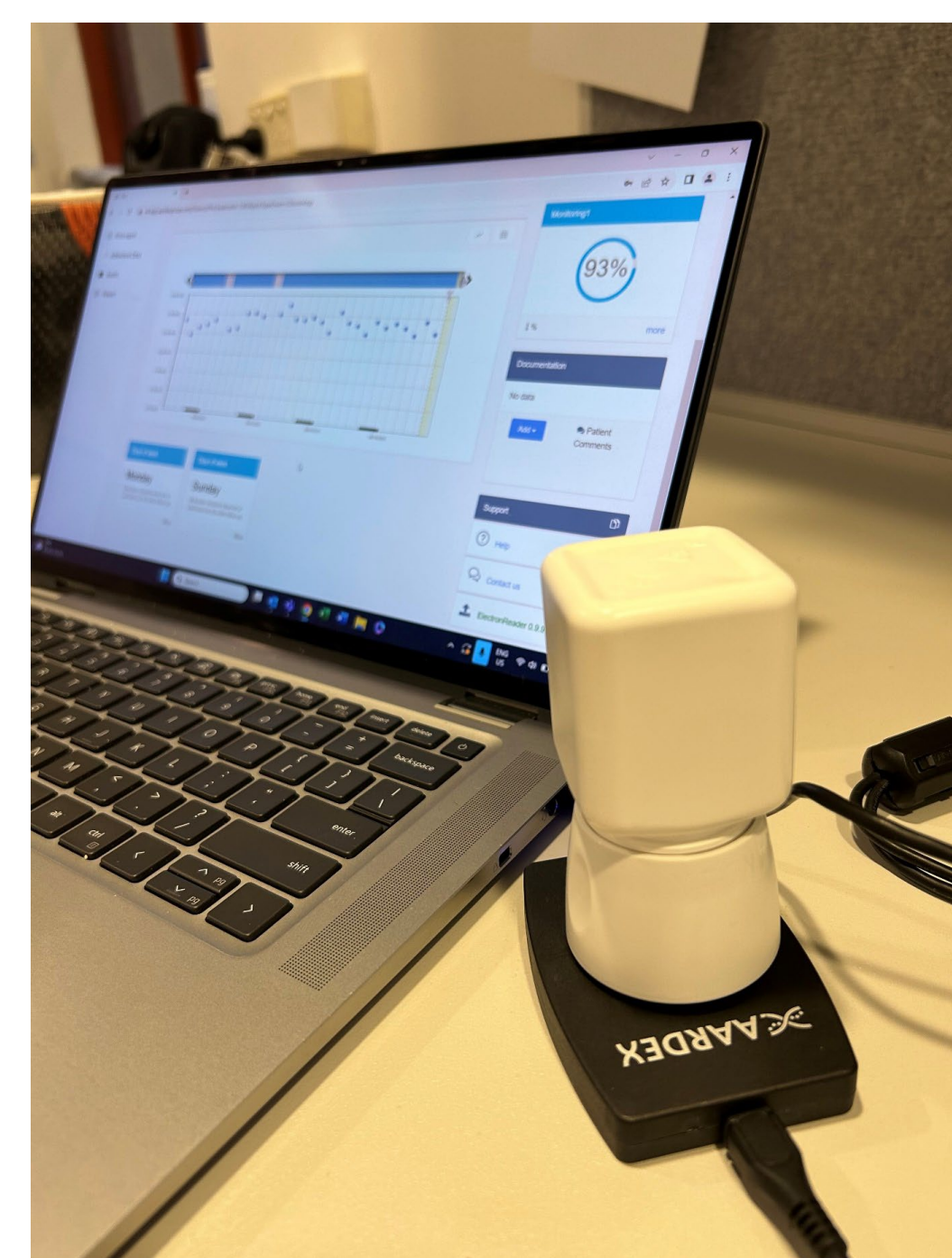
Figure 2. Activation of the MEMS SmartCap® using the MEMS Reader and the adherence dashboard on the MEMS software.
